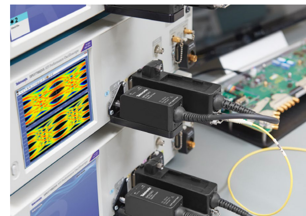
DP070E Series Optical probes using the TekConnect channel on a DP07002SX ATI Performance Oscilloscope.
